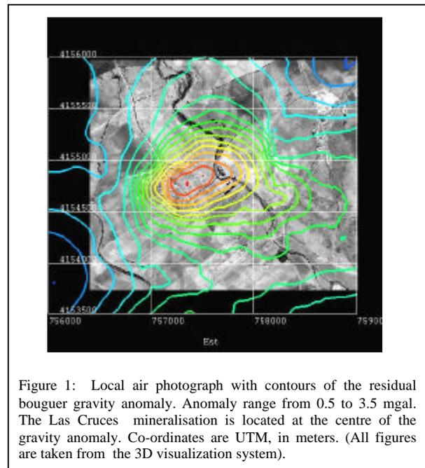
Figure 1: Local air photograph with contours of the residual bouguer gravity anomaly. Anomaly range from 0.5 to 3.5 mgal. The Las Cruces mineralisation is located at the centre of the gravity anomaly. Co-ordinates are UTM, in meters. (All figures are taken from the 3D visualization system).
