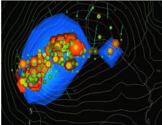
Figure 5: Plan view of 3D conductor interpolated from TEM soundings (blue isosurface encloses conductivities greater than 0.4 siemen). Drill hole traces show high copper grades as red and low green to blue. The diameter of each drill hole is linearly proportional to the measured core densities. Contours represent the residual gravity anomaly as shown in figure 1.
