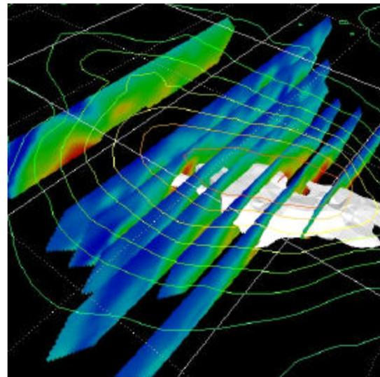
Figure 2: Oblique view of 2D inverted IP sections (blue low phase, red high phase) and intersecting white lens of high copper grades (>10%) interpolated from drill assays. Contours are the residual gravity contours shown in figure 1. Grid lines are 1km square and at ground level.
