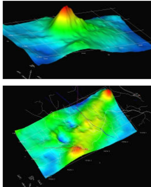
Figure 4: Top perspective surface is the observed residual gravity anomaly used for inversion modelling. (blue -0.5 to red 3.0 mgal). The lower perspective surface shows the difference between the gravity anomalies derived from forward modelling of the Vulcan density distribution (figure 3) and the observed anomalies. The SW-NE gravity ridge is the principal remaining anomaly.
